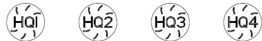
FIGURE 1. Head identification for HurriQuake® Nails, HQ1: 2-1/2x0.113 inch, HQ2: 2-1/2x0.131 inch, HQ3: 3x0.113 inch, and HQ4: 3x0.131 inch.
