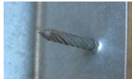
Photo 1: Stanley® BOSTITCH® Pneumatic Pins – C4S100BG, GC4S100BG & Pin Penetration through CFS Framing
